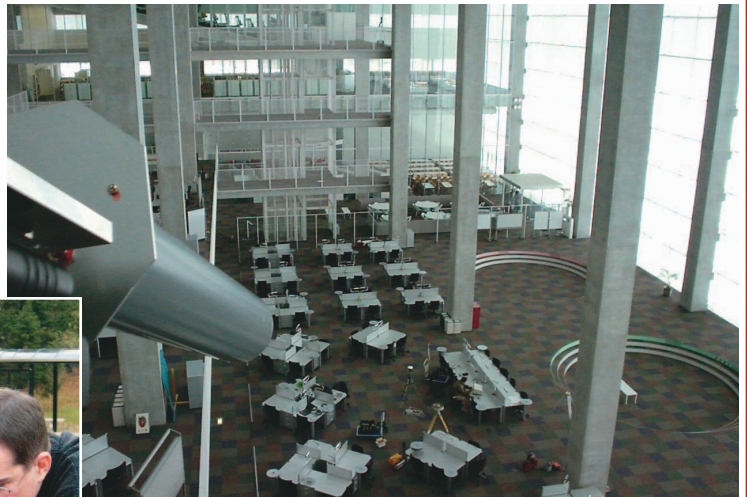
Indoor tests identified multipath effects and the opportunity to use a GPS retransmitter as a signal source.
