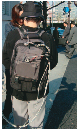
Backpack equipment for Tokyo test included pseudolite receiver, mapmatching system, and an audio interface.
