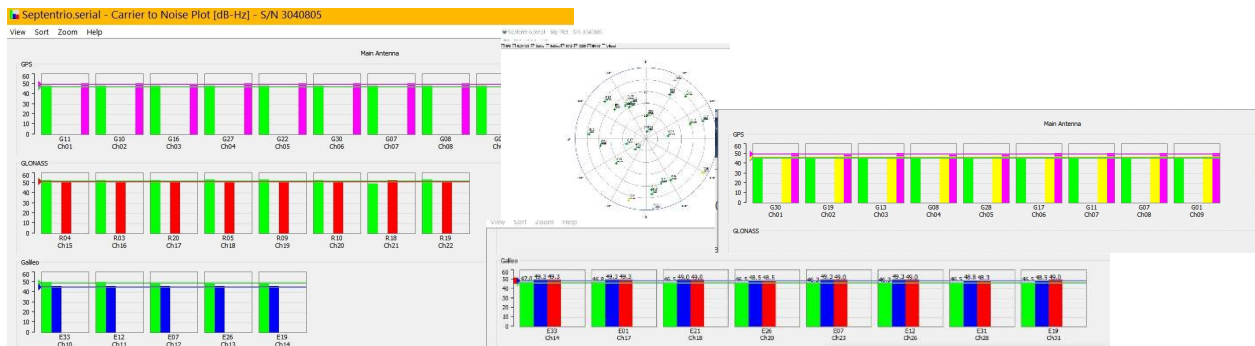
Septentrio receiver with dual and triple frequency GPS, GLONASS and Galileo simulated signals
